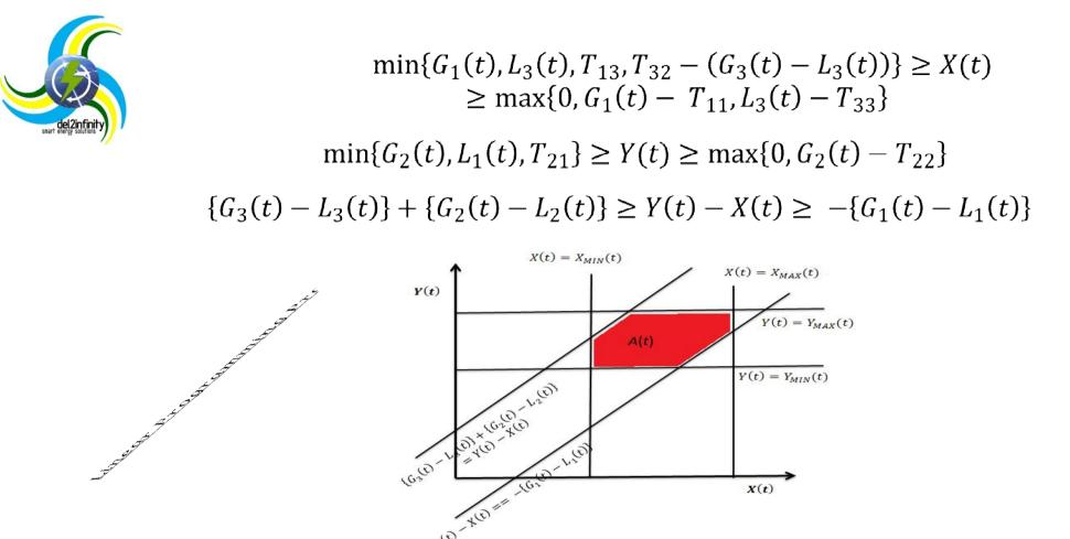
A(t) depends on the each value of  $G_1$ ,  $G_2$  and  $G_3$  but not on the sum of its values i.e.  $G_1 + G_2 + G_3$ . Interestingly since it is a variable generation and A(t) is not constant but to get the +ve value of A(t) we need a prediction of  $G_1$ ,  $G_2$  and  $G_3$  separately but not as a sum or aggregation of those values.
